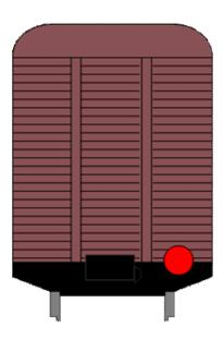
The reflective disc shall have a diameter of  $185\,$  mm with a red circle diameter of  $140\,$  mm.
